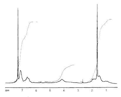
Fig. 2. 500 MHz <sup>1</sup>H NMR spectrum of PFNEMA-b-PSt-b-PFNEMA prepared by ATRP.
