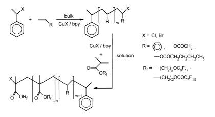
Scheme 1. Synthesis of fluorocarbon/hydrocarbon diblock copolymers by ATRP.
