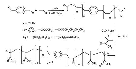
Scheme 2. Synthesis of fluorocarbon/hydrocarbon triblock copolymers by ATRP.
