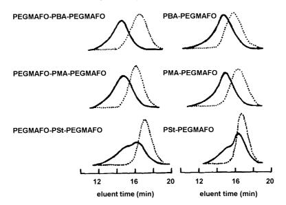
Fig. 3. GPC traces of macroinitiators (--) and the produced block copolymers (--) described in Table 3.
